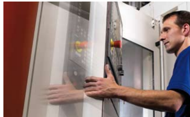
■ Practical feature: the ergonomic operating panel is integrated into the guard panels.
